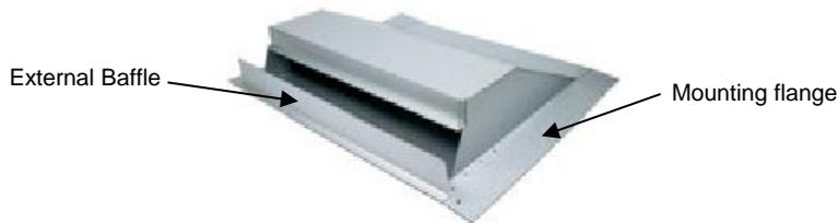
**TAMCO Off-Ridge Roof Vent with Baffle** Minimum 26 ga. ASTM A792 AZ50 (non-HVHZ only) or ASTM A653 G90 steel off-ridge static roof ventilator with integrated baffle offset from the intake. Vent dimensions are 24" wide x 4-1/4" high and is available in nominal lengths of 4-ft, 6-ft, 8-ft and 10-ft. Material shall conform with FBC Section 1507.4.3 (non-HVHZ) and 1517.6 (HVHZ).
